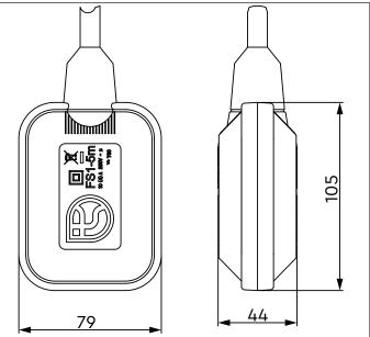
Note: For control of a pump with a full load in excess of 4 Amps, the Floating Switch must be wired through a connector relay.
