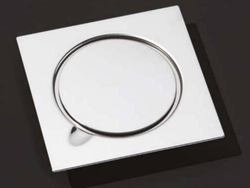
Code: FD150.7 Size: 15 x 15 Material: AISI 304 Model: screwed grating and centrally screwed cover, which allows continuous drainage even when the cover is mounted Outlet size: 103 mm / 4 inches
